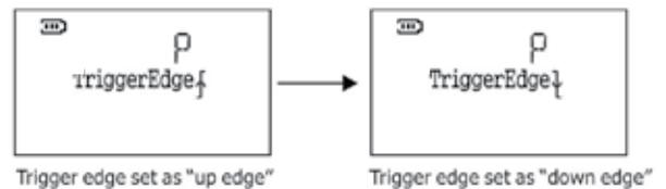
When trigger edge setting is set to “up edge”. The flash will occur on the leading edge of the input pulse (when delay setting is zero).
