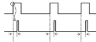
When trigger edge setting is set to “down edge”. The flash will occur on the trailing edge of the input pulse (when delay setting is zero).
