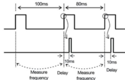
If the period of the external input is less than the setting of the delay time, the delay time is ignored and the DT-366 flashes as if the delayed time equals 0.
