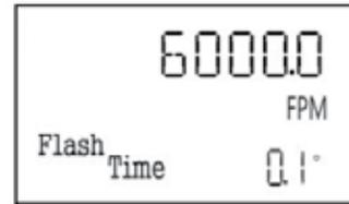
To set the flash pulse duration while in the modifiable mode; press “+” key, or turn the dial in the clockwise direction to increase the flash pulse duration by 0.1° increments.
