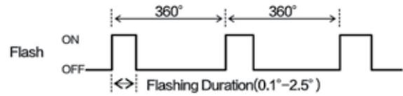
When the flash duration is lengthened, the brightness of the flash will be increased, however the image of the target object may appear slightly out of focus. When the flash duration is shortened, the brightness will be decreased, yet the image of the target object will become more focused.
