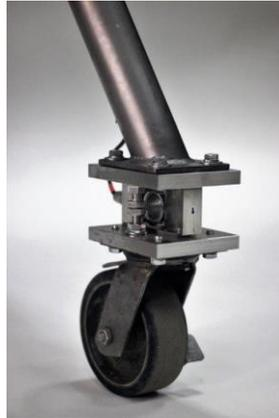
The addition of top and bottom plates enables a weighing module to be created that inserts directly in place of the existing caster, without any modification required to the caster or the vessel frame.
