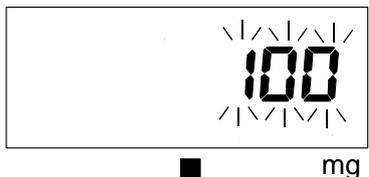
[ 4 ] Press the
