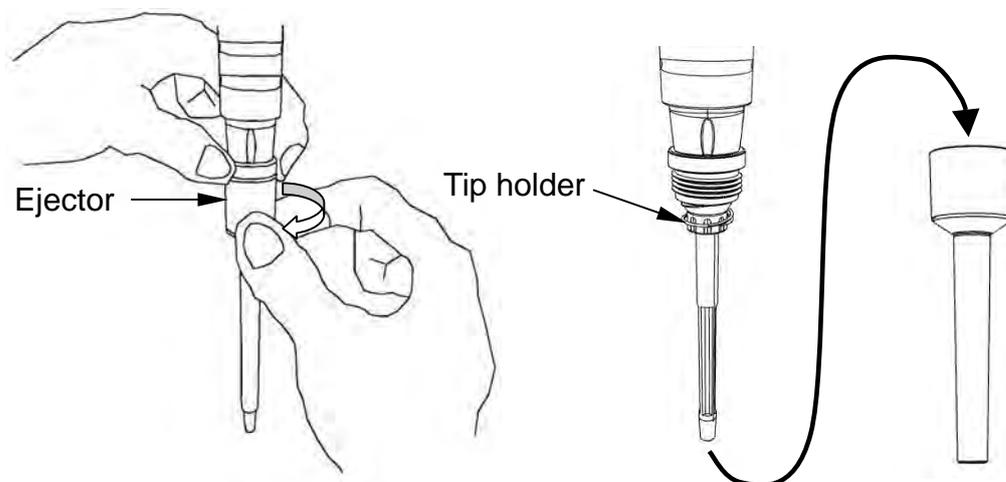
Regularly clean the tip holder about once every half a year to a year, depending on the frequency used. Regularly confirm the pipette accuracy.
