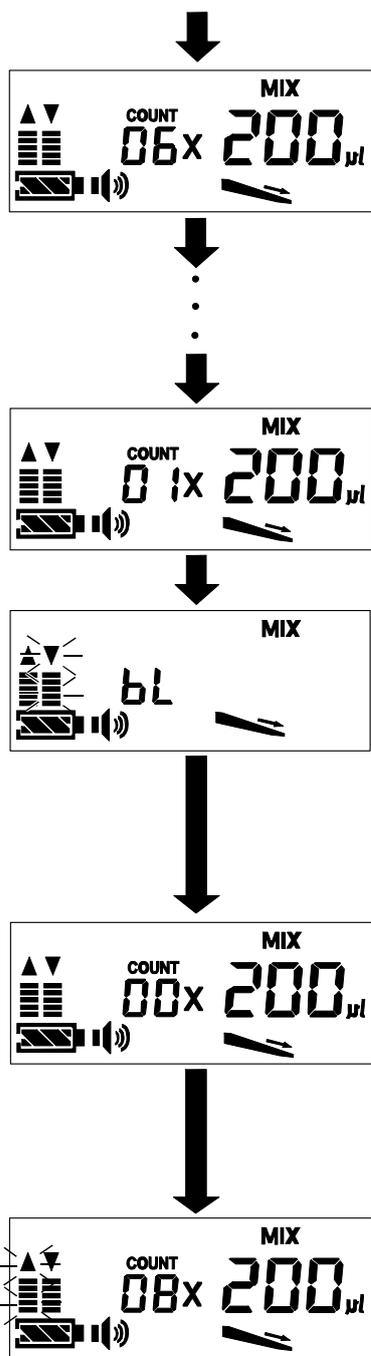
[ 3 ] The pipette executes the set count of aspirating-dispensing cycles by approx. 2/3 of the set mixing volume.
