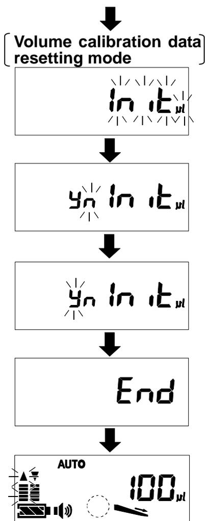
[ 3 ] Press the
