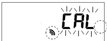
[ 3 ] Press the
