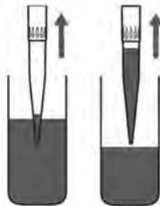
[ 2 ] Put the tip end into the receiving vessel and press the
