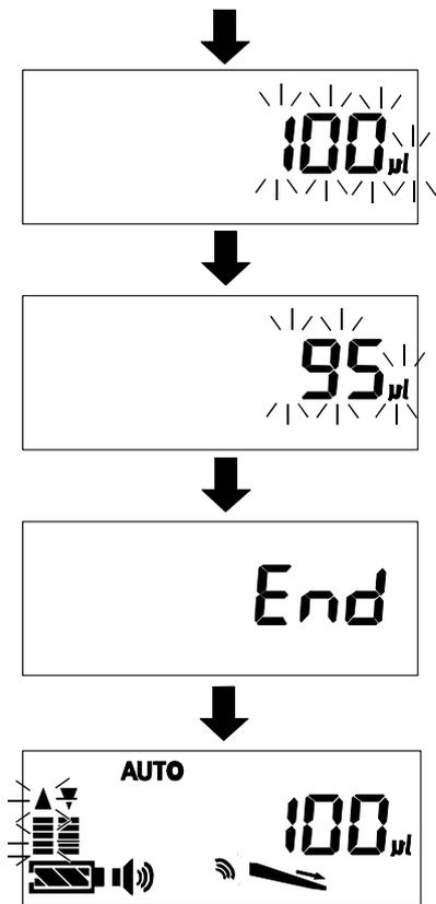
[ 3 ] Press the
