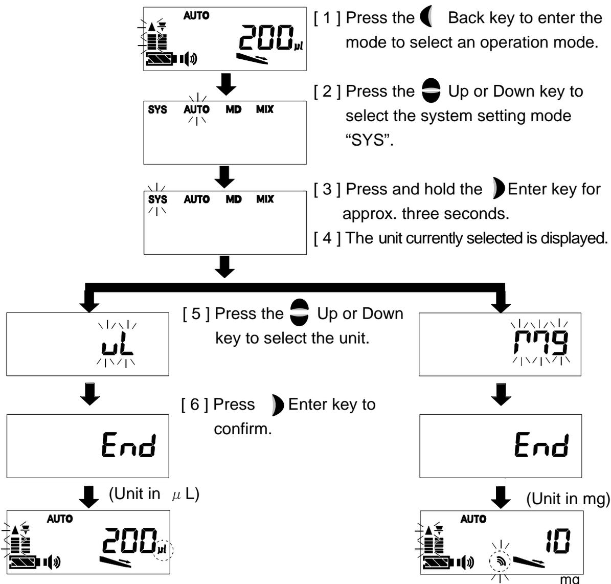
With the  $\mu$  L unit selected, the Notice mark is turned off while the  $\mu$  L unit mark lights up.
