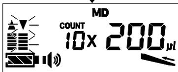
[ 2 ] Put the tip end into a receiving vessel and press the
