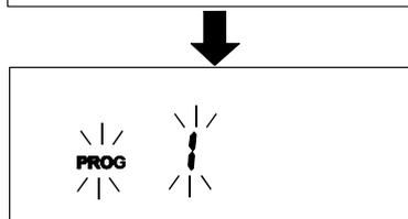
[ 1 ] Press and hold the
