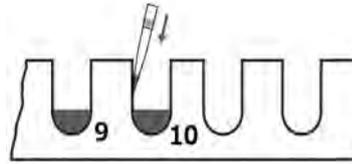
[ 5 ] Press the
