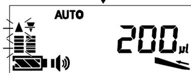
[ 1 ] Press the
