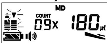
[ 3 ] In a similar manner, put the tip end into the next vessel and press the
