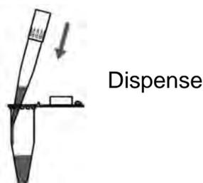
[ 3 ] Press the
