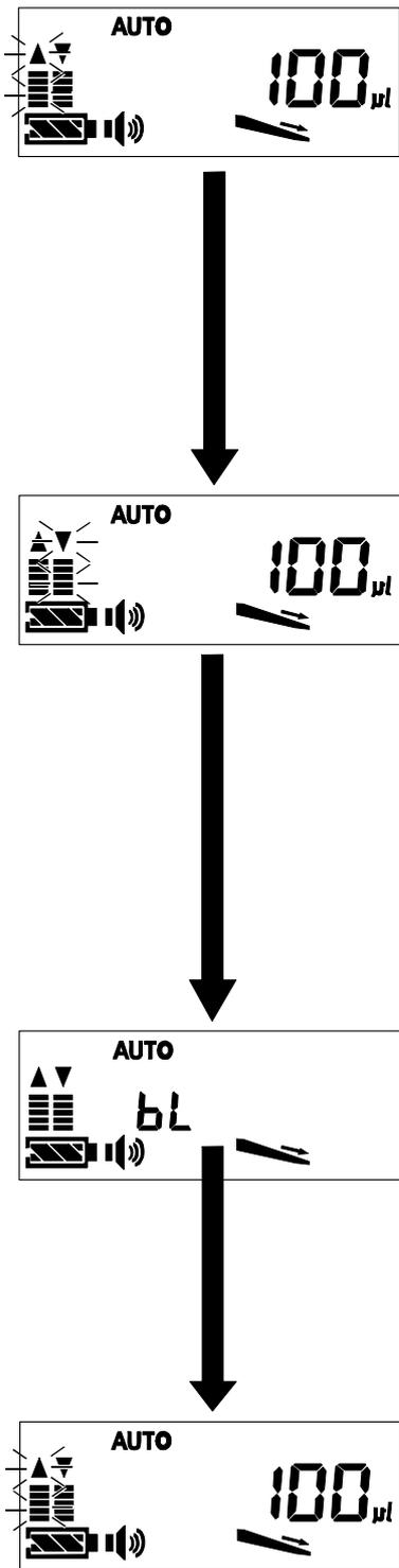
[ 1 ] Put the tip end into the liquid to be dispensed and press the
