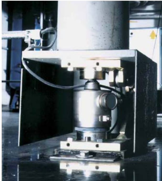
Figure F: 20,000 kilogram compression load cell and mounting hardware with installed heat shield.
