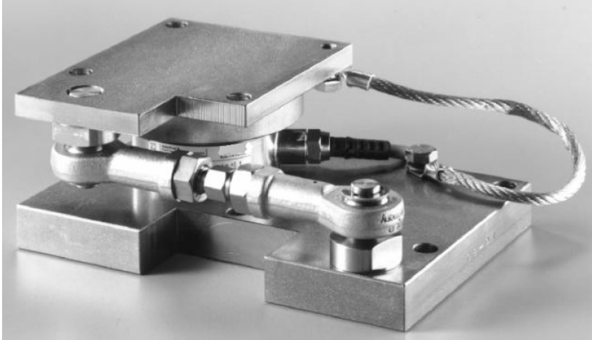
Figure G: A compression load cell mounting kit with side force protection. Top plate pictured above would mount to a tank leg and bottom plate to foundation or bottom supporting frame
