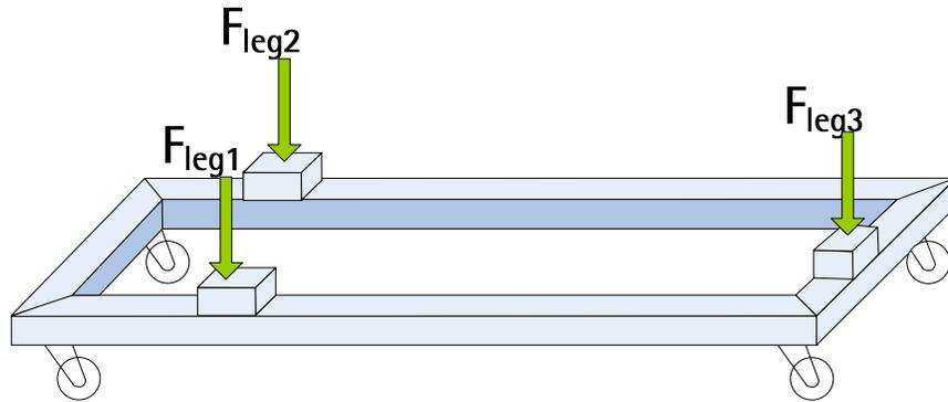
Figure 4: Correct portable tank system design for a 3-legged tank
