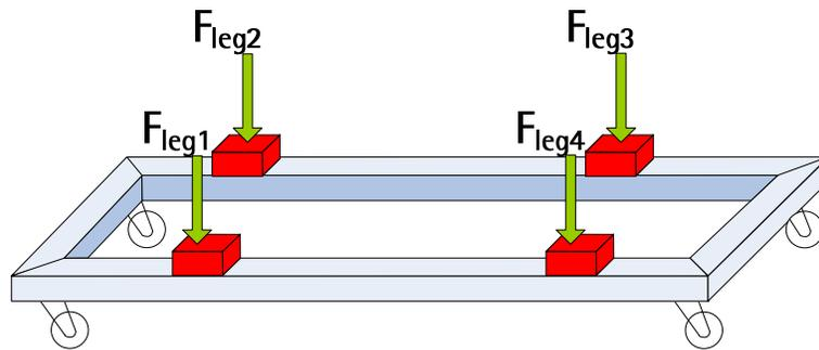
**Figure 1: Incorrect four-legged portable tank system**
