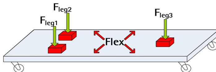
Figure 3: Incorrect portable tank system with steel plate
