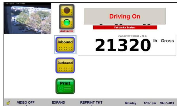
Once a "TRUCK OFF SCALE" message is displayed and the Loop no longer senses the vehicle, and motion is slowing, the FB2550 will display this message.
