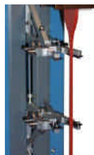
Extensometer arms open to engage with sample
