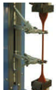
Extensometer arms closed and engaged with sample
