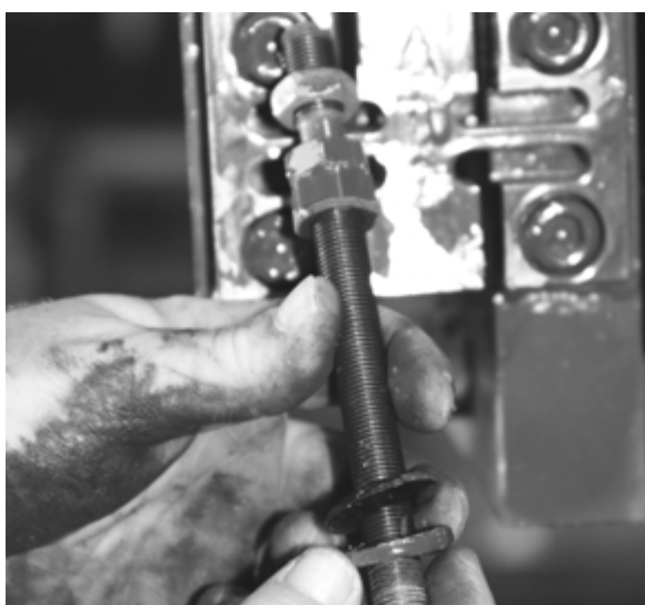
Figure 2-5. Remove Flexure Rod with Nuts and Washers
