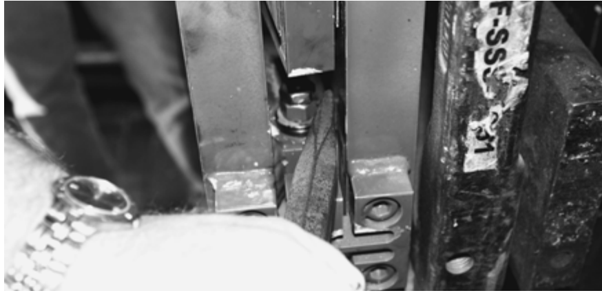
Figure 2-12. Centering the Load Cell Using a Chisel
