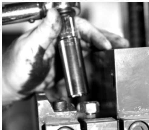
Figure 2-3. Removal of Hex Nut (Item #1 in Figure 2-2)
