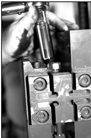
Figure 3-10. Remove Hex Nut
