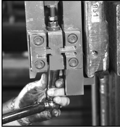
Figure 3-11. Remove Bottom Nut
