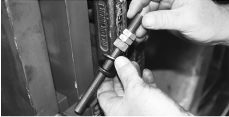
Figure 2-10. Install Spherical Washer Set
