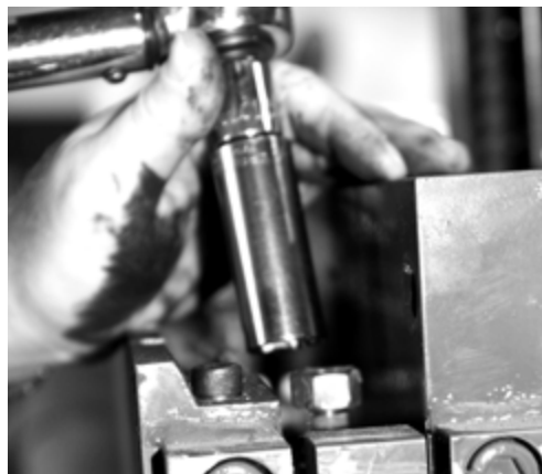
Figure 2-3. Removal of Hex Nut (Item #1 in Figure 2-2)
