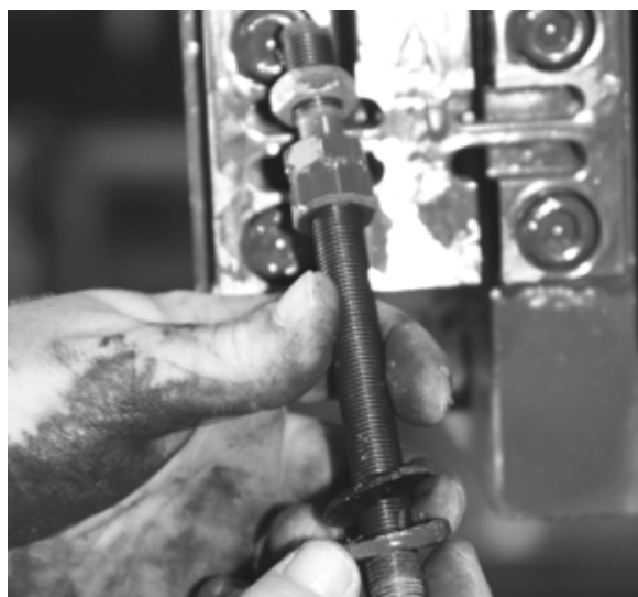
Figure 2-5. Remove Flexure Rod with Nuts and Washers
