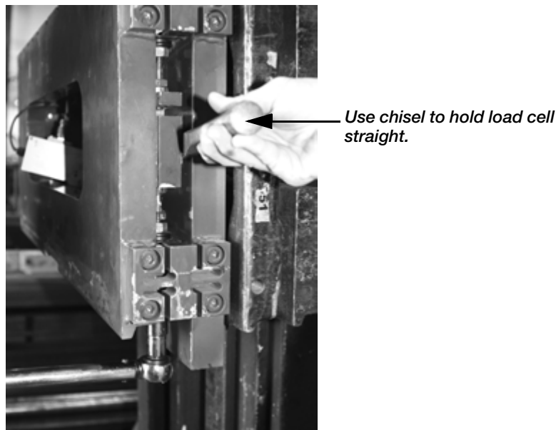
Figure 2-9. Use Chisel to Hold the Load Cell in Straight
