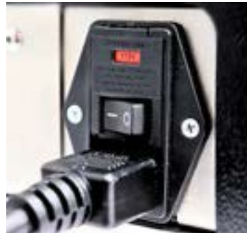
The Main Power switch.
