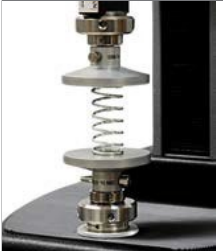
Proper alignment of the test specimen.
