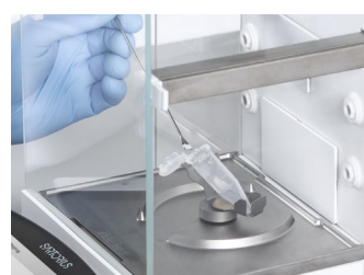
YSH14-3 Reaction Tube Holder (up to 2 mL)
