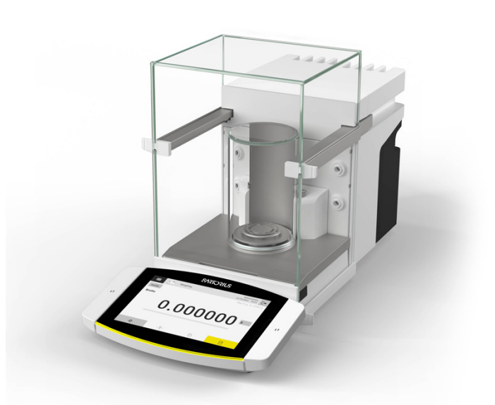
Figure 5: Cubis® II MCA66S with automated inner draft shield.
