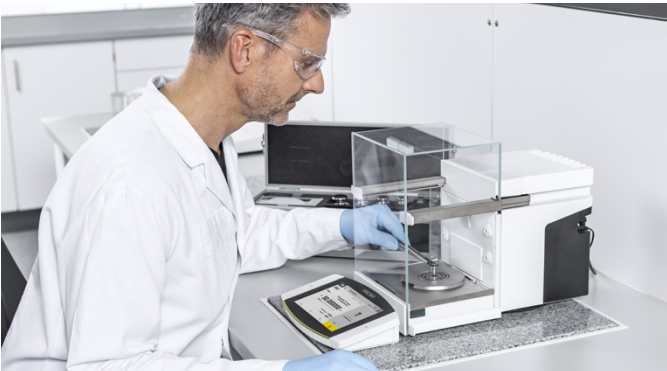
Figure 1: Determining the minimum sample weight on a Cubis® II MCA66S according to USP Chapter 41.
