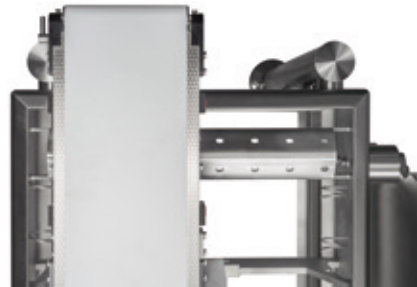
Example: no hollow spaces, easy inspection
